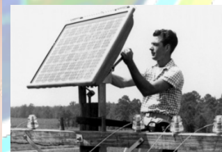
Test of a 6% efficient solar panel, 1959
